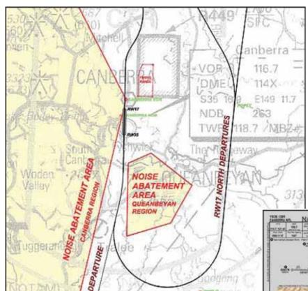
Naverus and Qantas worked with Canberra ATC to thread RNP procedures through the existing airspace constraints
